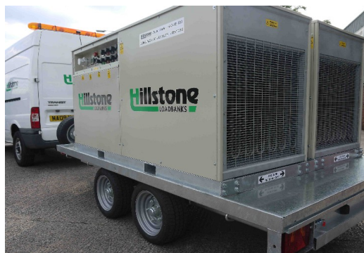
1200KW trailer mount unit illustrated ( 2 x 600KW modules )
